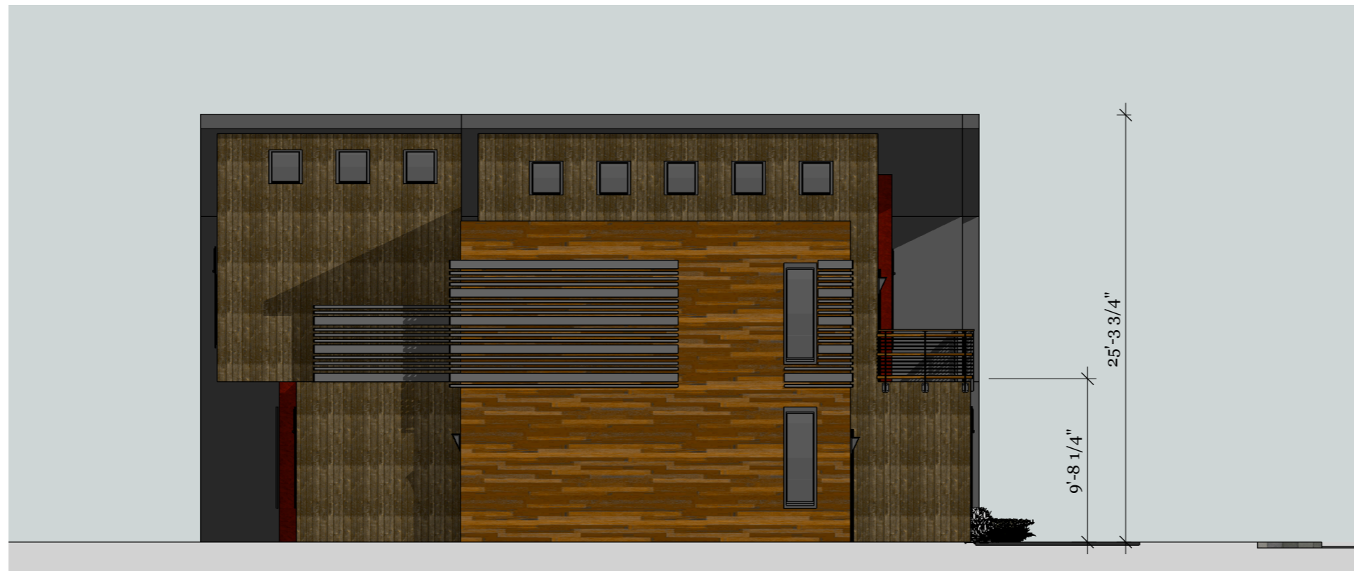
A 1 Elevation - Left Side 1/8" = 1'-0"
